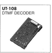
Provides DTMF decode capability with code squelch and pager operation.
